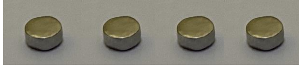
Figure 1. Sample of nickel-chromium alloy with a diameter of 5mm and a thickness of 2mm
