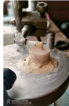
**Fig. 4:** Polishing with diamond paste
