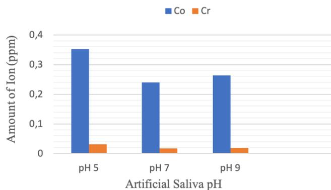
**Figure 5.** Comparison of released Co and Cr ion from 5  $\mu$ m silver coated CoCr alloys immersed in artificial saliva with various pH
