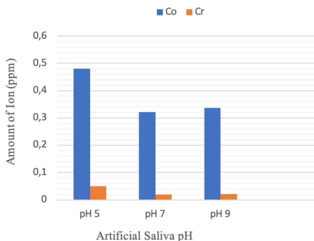
**Figure 6.** Comparison of released Co and Cr ion from uncoated CoCr alloys immersed in artificial saliva with various pH
