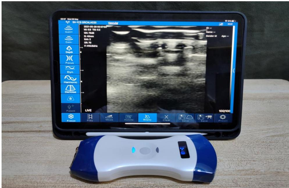
**Fig.1** Wireless Dual Head Ultrasound Probe (HOCHEY MEDICAL, Anhui, China)
